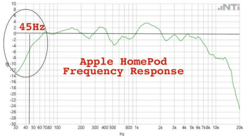
APPLE'S HOMEPOD TRAILS OFF IN AROUND 45HZ IN THIS EXAMPLE, BUT EACH PLACEMENT CAN VARY
