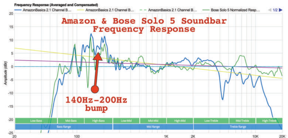
Soundbar examples from Amazon and Bose show 'mid-bass' bump; common in this audio speaker form factor
